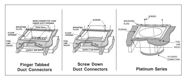
Figure 9. Duct Connector
